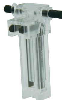
Figure 2: A carbon electrode zeta potential cell, usable after several hundred measurements
