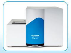
The PSA300 is a turn-key, static image analysis solution. Seamless integration of powerful particle characterization software and an automated microscope with a high resolution camera creates an intuitive, easy-to-use imaging workstation. It features a dry dispenser for proper particle dispersion and a four position autosampler. Minimum intervention by the operator still yields maximum detail in the results.
