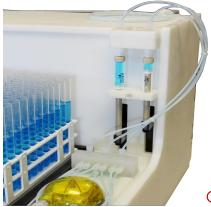
Spikes sample with internal standards Performs multiple dilutions Prepares calibration and QC standards Serial dilutions and aliquot transfers Consistent and precise reagent addition
