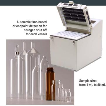
Measurements - Concentration / Evaporation vessels in 500  $\mu$ L, 1 mL, and direct to a GC Vial or to dryness
