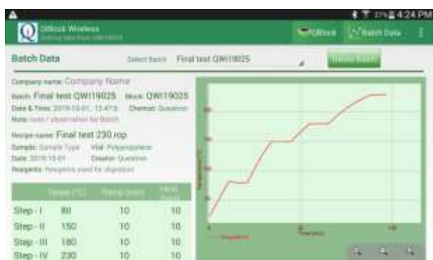
Touch screen display of heating profile
