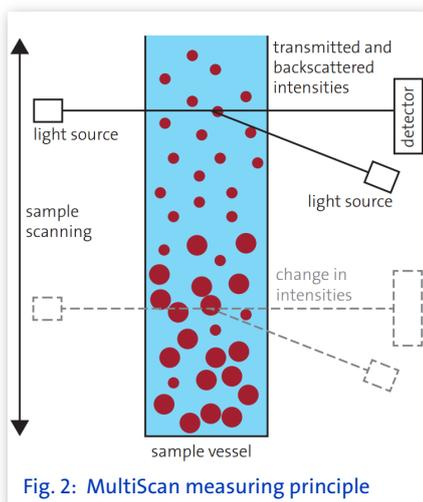
Fig. 2: MultiScan measuring principle
