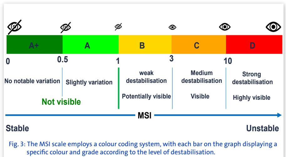
Fig. 3: The MSI scale employs a colour coding system, with each bar on the graph displaying a specific colour and grade according to the level of destabilisation.
