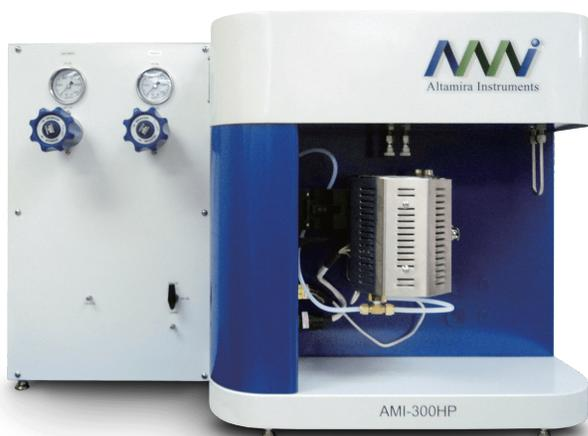
AMI-300HP is a high temperature and high pressure chemisorption analyzer developed on the basis of AMI-300 to meet higher scientific research needs. In addition to the basic experiments that can be done with AMI-300, the performance of the catalysts can be further investigated at high pressures. This type of instrument can be tested at atmospheric pressure up to 100bar.
